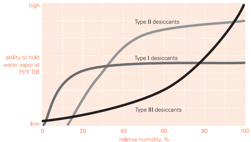
Figure 1. Typical desiccant isotherms
