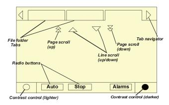
The file folder tabs across the top of the screen are used to select the various display screens.
