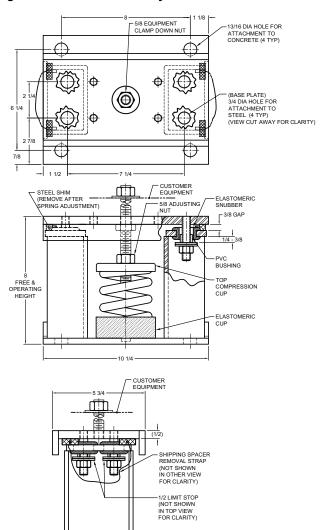
Install the optional seismically rated isolators at each mounting location specified in section "Seismic Isolator Mounting," p. 41. See Figure 15 for correct orientation, and Figure 16 for installation reference.
