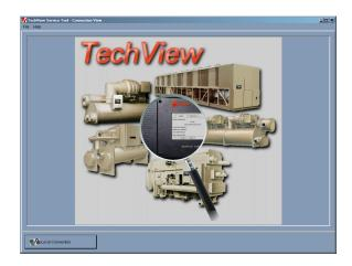
TechView™ is the PC (laptop) based tool used for servicing Tracer® CH530. Technicians that make any chiller control modification or service any diagnostic with Tracer® CH530 must use a laptop running the software application "TechView." TechView is a Trane application developed to minimize chiller downtime and aid the technicians understanding of chiller operation and service requirements.
