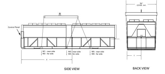
Figure 10. Lifting the unit (packaged and remote) — 39 to 45 foot base
