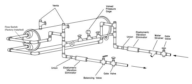
Install field-supplied pressure components as shown in Figure 26, p. 50. Locate pressure gauges or taps in a straight run of pipe; avoid placement near elbows, etc. Be sure to install the gauges at the same elevation on each shell if the shells have opposite-end water connections.
