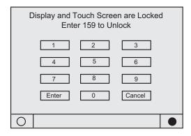
**Note:** This feature is provided to avoid unintended actuations of the keypad, which can occur due to ice build-up on the DynaView's exterior surfaces. Also be aware that at extremes of temperatures, the LCD display screen will change its contrast from the optimal adjustment made at more normal temperatures. It can appear washed out or blacked out. Simply pressing the lower right contrast control on the screen will return the display to readable condition.
