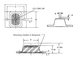
can be reduced by elastomeric vibration eliminators. Spring isolators are not recommended for non-seismically rated applications. Consult an acoustical engineer in critical sound applications.
