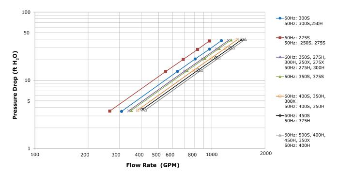
Figure 24. Evaporator water pressure drop, 3-pass evaporator, 120 to 250 tons
