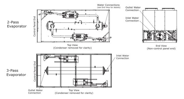
Figure 20. Evaporator pass configurations, 3 or 4 compressor units
