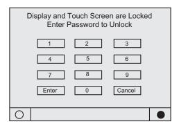
Note: The DynaView display and Touch Screen Lock screen is shown below. This screen is used if the Display and touch screen and lock feature is enabled. Thirty minutes after the last keystroke, this screen is displayed and the Display and Touch Screen is locked out until the sequence "159 <ENTER>" is pressed.
