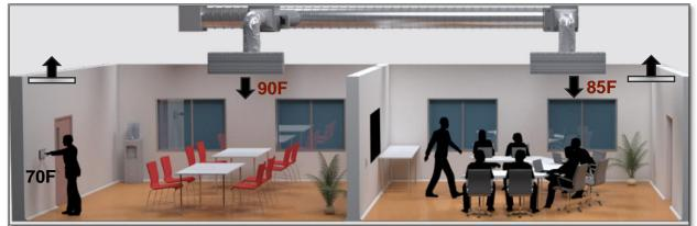
Draw Thru fans -UL limit of 104F air for motor -More critical today for units with ECM fans
