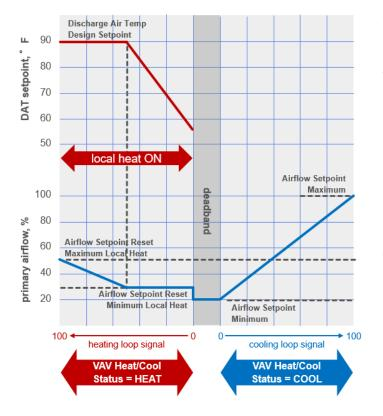
VAV terminal unit control sequence with SCR electric or modulating hot-water heat (i.e., "dual max sequence")
