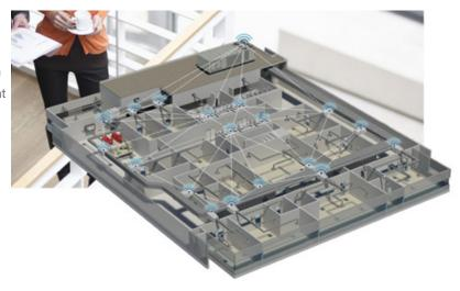
The Air-Fi® Wireless Communications Interface (WCI) enables wireless communications between system controls, unit controls, and wireless sensors for Trane® control products that use the BACnet® protocol. The WCI replaces the need for communications wire in all system applications.
