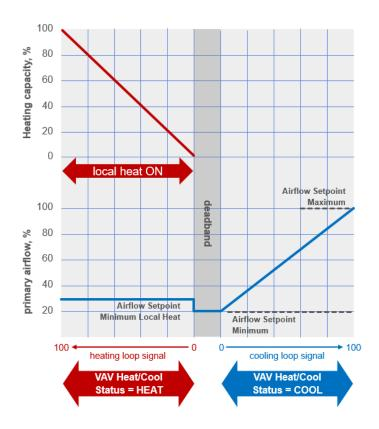
VAV terminal unit control sequence with staged electric or two-position hot water heat
