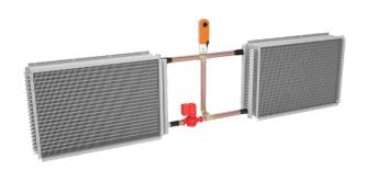
Coil loops, sometimes called coil run-around loops, have two or more finned tube coils that are piped together in a closed loop. A fluid is circulated by a pump between the coils to transfer sensible heat from one air stream to another. The fluid is often water mixed with a freeze inhibitor like glycol.
