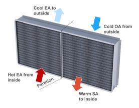
A heat pipe is like a coil loop but not quite as flexible. The typical configuration requires the airflows to be side-by-side, as shown here. Each assembly contains multiple heat pipes. Each is an independent sealed tube filled with a heat-transfer fluid—often refrigerant. A partition divides the heat pipe into separate "evaporator" and "condenser" sections.
