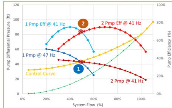
Efficiency-based pump staging
