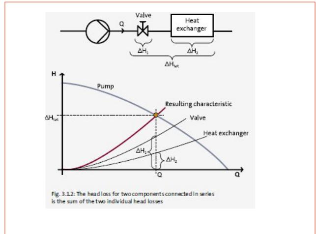
Fig. 3.12: The head loss for two components connected in series is the sum of the two individual head losses
