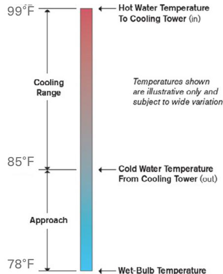
defines the cooling capability of the cooling tower. The figure above provides a visual representation of the relationship between range and approach.<sup>2</sup>
