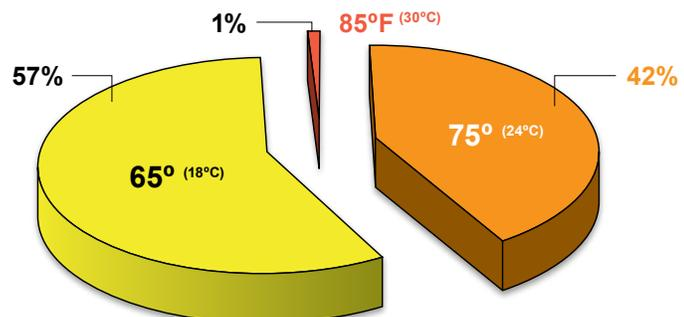
In addition to part-load assumptions, the IPLV calculation uses weighted national averages of numerous factors that may or may not correspond to a specific building's profile. These factors include weather data from 29 cities across the United States and building types based on a Department of Energy study of buildings. Additional weighted average factors include operational hours (for operations with chiller plants only) and chiller plants both with and without an economizer.
