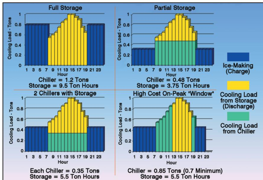
Figure 1: Chiller/storage selection (1 ton peak load, 9.5 total ton hours).
